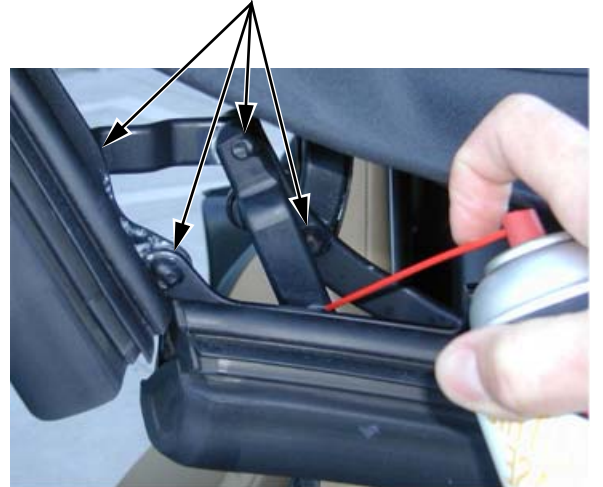
TOP FRAME PIVOT POINTS (FROM OUTSIDE)
