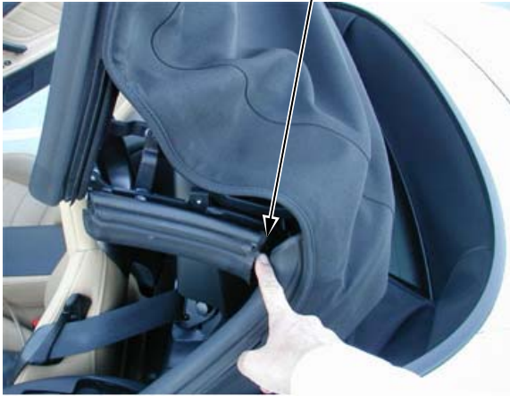
END OF THE CONVERTIBLE TOP FRAME AND DOOR GLASS WEATHERSTRIP
